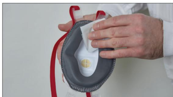
If the respirator is to be used for more than one shift the face seal must be cleaned at the end of each shift using a 3M™ Face Seal Wipe 105. The respirator should be stored in a sealed, clean bag or container between uses.
